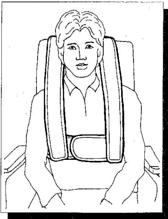
Self-release with "hook & loop" in front.
